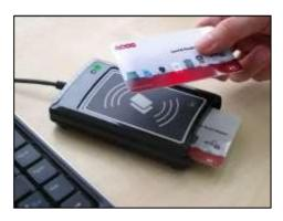
ACR1281U-C1 DualBoost II is the second generation of ACS's ACR128 DualBoost Reader. It is a dual interface reader that can access any contact and contactless smart cards following the ISO 7816 and ISO 14443 standards. ACR1281U-C1 enables one to conventionally integrate both separate and independent applications for contact and contactless technologies into one device and one card.
